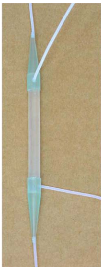
Fig. 2. Image of the countercurrent microextraction chamber.
